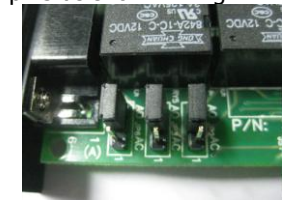
Fig. 7 Jumper setting for ACTIVE OPEN
