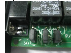
Fig. 6 Jumper setting for ACTIVE CLOSE
